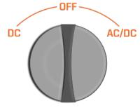
**LEFT POSITION:** All DC ports (12V DC sockets, Basecamp LED Light ports, and the USB ports) on, otherwise referred to as DC ONLY mode. This will also activate the LCD Display.
