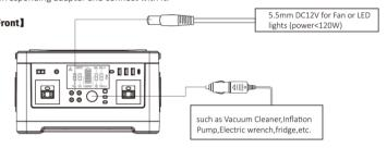
**Note:** The 12V DC output voltage is range between 9V~12.6V, maximum output current is 12A. DC output voltage drops while battery capacity drops due to chemical characteristics of the battery. If your appliance is not built-in input voltage stabilizing function, it may shutdown when input voltage is too low, please unplug your device from the unit in time And please charge the unit in time.
